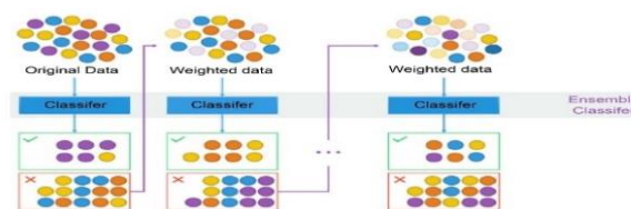
Fig. 5. AdaBoosting model architecture (1).
